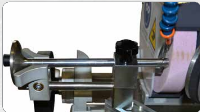
Valve end refacing by means of the universal support on issue: this means a perfect equalization of the engine valve height.
